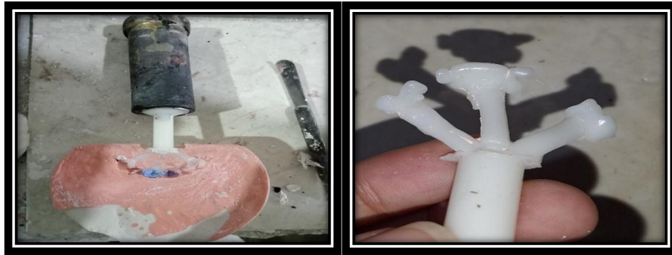
Figure 1.21. Failure Results (low temperature, sprue placement) (Source: Primary data, 2022)
