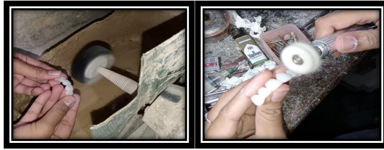
Figure 1.19. polishing (Lathe brush and Rag wheel) (Source: Primary data, 2022)
