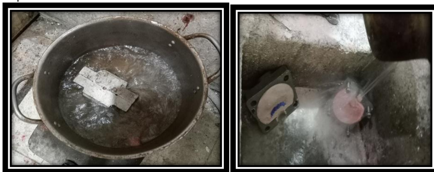
Figure 1.12. Boiling out process (cooking cuvettes and watering)(Source: Primary data, 2022)
