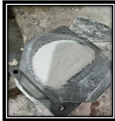
Figure 1.11. Upper Cuvette Flasking(Source: Primary data, 2022)
